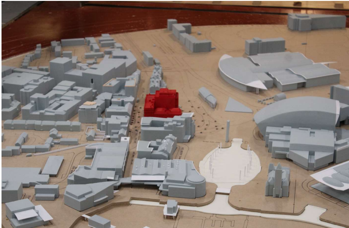
Figure 11: Proposed Development with Existing Surrounding Buildings and Mitigation Measures (Configuration 2) – View in the Wind Tunnel from the south
