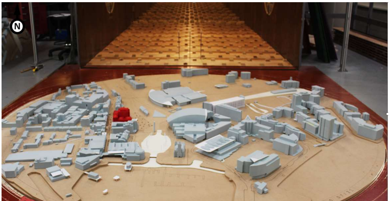
Figure 2: View from the south of the Proposed Development (in red) with existing surrounding buildings (in white) in wind tunnel
