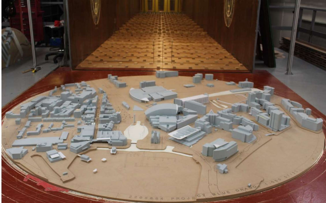
Figure 8: Existing Site with Existing Surrounding Buildings (Configuration 1) - View in the Wind Tunnel from the south
